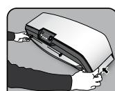
The Titan™ laminator has integrated carry points for safe and easy movement of the laminator – push in the flaps on both ends of the laminator to access them.
