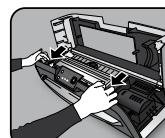
To open the belt-drive mechanism, Pull the 2 cam levers forwards, on each side of the mechanism. The upper carriage can now be lifted upwards from the front. Lift the carriage and open fully until it stops in the rest position.
