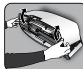
Lift the top cover with both hands. The laminating engine and belt-drive mechanism will be visible.
